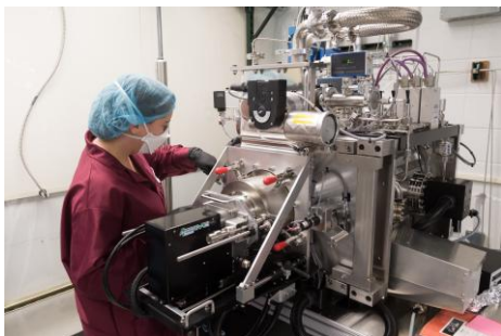
Fig. 7. Bias target deposition system used to deposit mixtures of several oxides to create ternary and quaternary thin films. In this process, metal targets are biased to accelerate Ar ions into the target and sputter the target in a reactive oxygen atmosphere.
