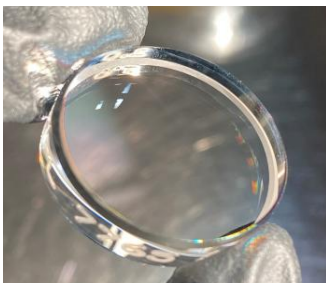
Fig. 6. Multilayer mirror consisting of a stack of GeTiO and SiO 2 layers, designed for high reflectivity at 1064 nm wavelength.
