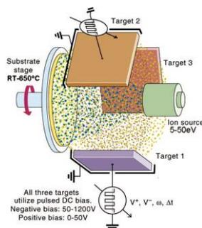
interferometer cavities of gravitational wave detectors. This project will offer the REU student opportunities to learn how to grow thin film metal oxides by sputtering. The REU student will learn how to characterize the materials by ellipsometry and spectrophotometry to analyze their optical properties. The REU student will be exposed to interferometry, spectroscopy methods and x-ray diffraction to determine mechanical and structural properties of the thin films.
