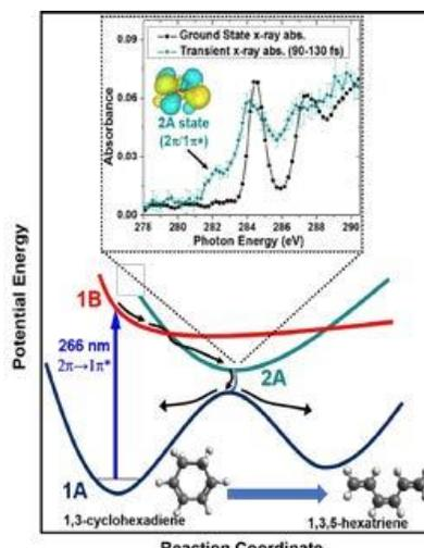
**Figure 6:** Direct fs identification of the transition state 2A, arrow, for cyclohexadiene ring opening.
