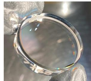
**Figure 4.** Multilayer mirror consisting of a stack of GeTiO and SiO<sub>2</sub> layers, designed for high reflectivity at 1064 nm wavelength.
