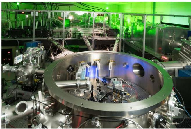
**Fig. 1.** Target chamber for the interaction of ultrahigh intensity laser pulses with materials.
