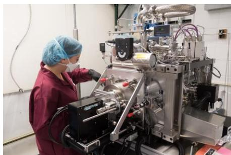
**Figure 3.** Bias target deposition system used to deposit mixtures of several oxides to create ternary and quaternary thin films. In this process, metal targets are biased to accelerate Ar ions into the target and sputter the target in a reactive oxygen atmosphere.
