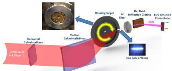
**Figure 1:** Schematic of table-top EUV laser. An optical laser beam is focused into a selected solid rotating target to generate a line focus plasma from which an EUV laser beam is generated.
